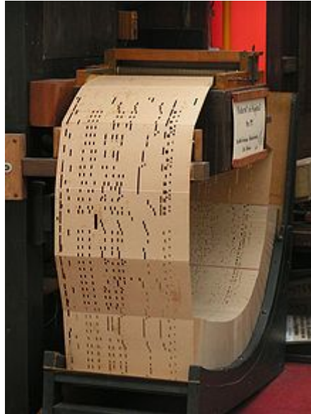
Punched card system of a music machine, also referred to as Book music
