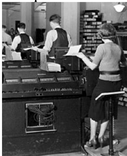
IBM punched card Accounting Machines at the U.S. Social Security Administration in 1936.
