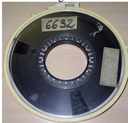
Half-inch (12.7 mm) magnetic tape, originally written with 7 tracks and later 9-tracks
