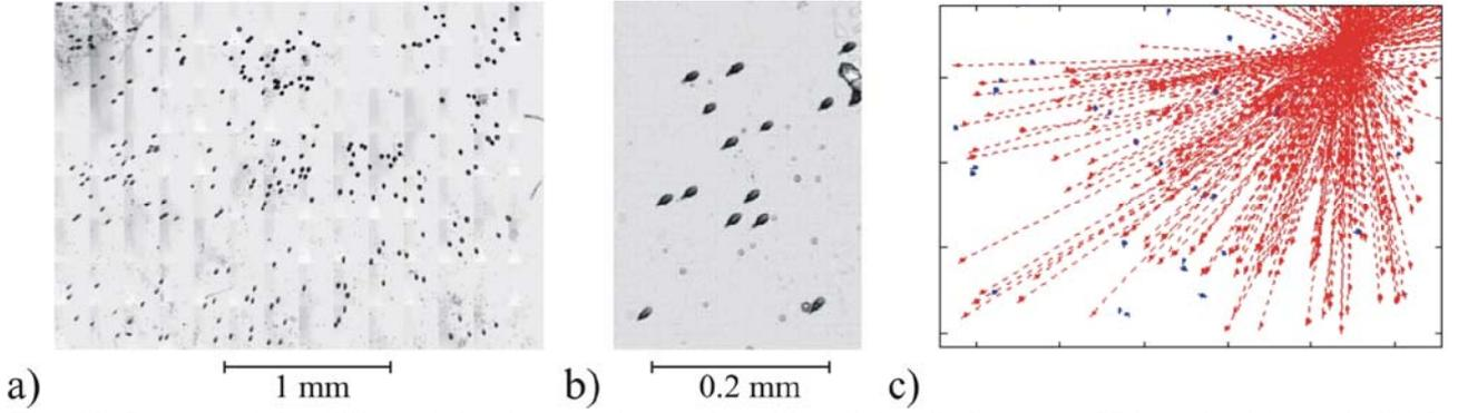
**Fig. 10.** Pattern of the filling of the detector by tracks with a “giant” cluster of 276 tracks (a); an individual fragment of the pattern (b); the diagram of track directions (c). Mean energy per particle in the cluster (lithium or  $\alpha$ -particle) is of the order of 5 MeV.
